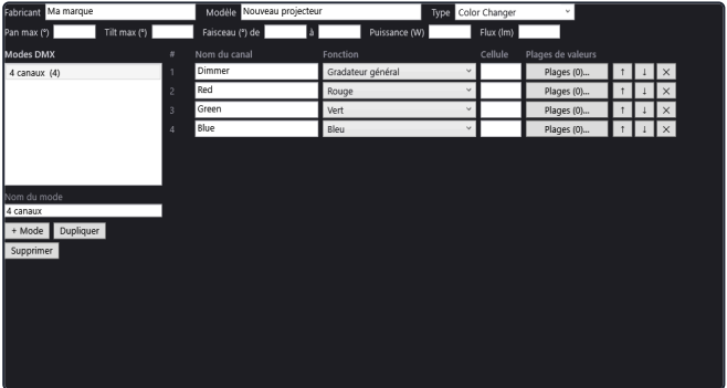
The fixture editor: modes, channels, functions, cells and value ranges.
